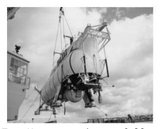
Tom Vetter and two fellow explorers fit in the tiny windowed sphere between the bathyscaphe's front legs. Everything else was for controlling buoyancy.
