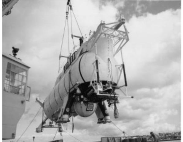
Tom Vetter and two fellow explorers fit in the tiny windowed sphere between the bathyscaphe's front legs. Everything else was for controlling buoyancy.
