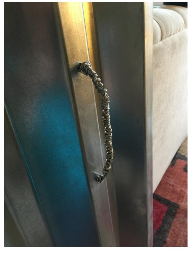
ing on the front, and loose wrapping twisted into a tail on the back. I did extra wrapping around the holes both front and back to act as ad hoc washers, and meet the ridigity spec. Took about half an hour to build this one.
